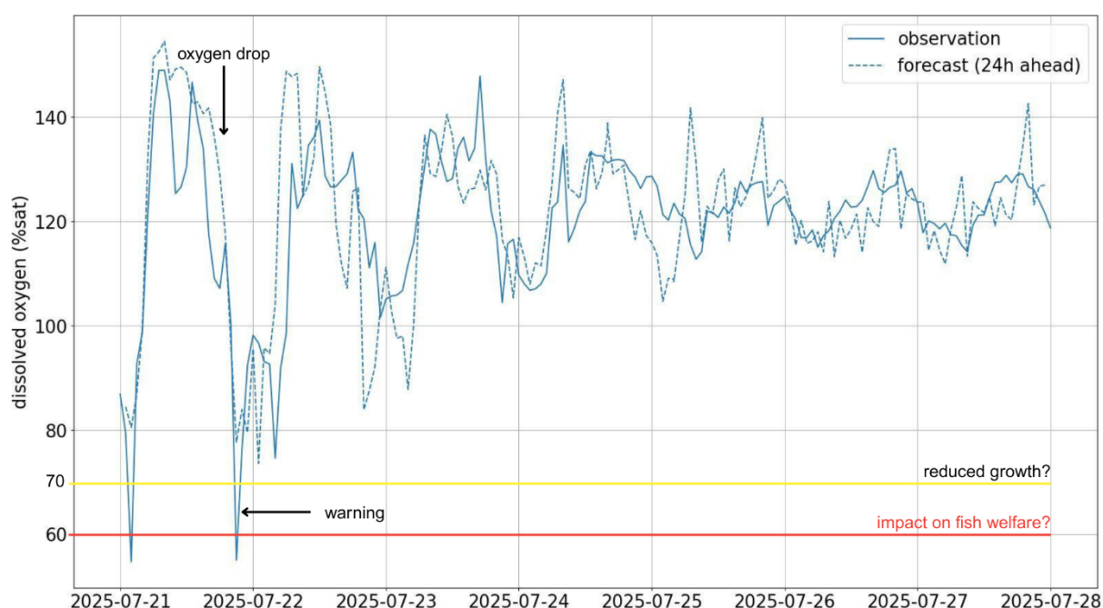
Figure 4. Example of a DO forecast time-series by BiOceanOr at a salmon farming site in Norway.
