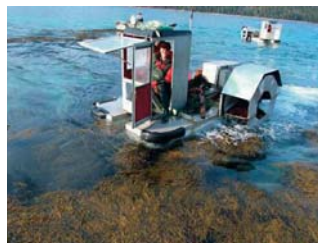
(3) Vessel with a paddle wheel cutter, used to harvest Ascophyllum nodosum in Norway © Sander.
